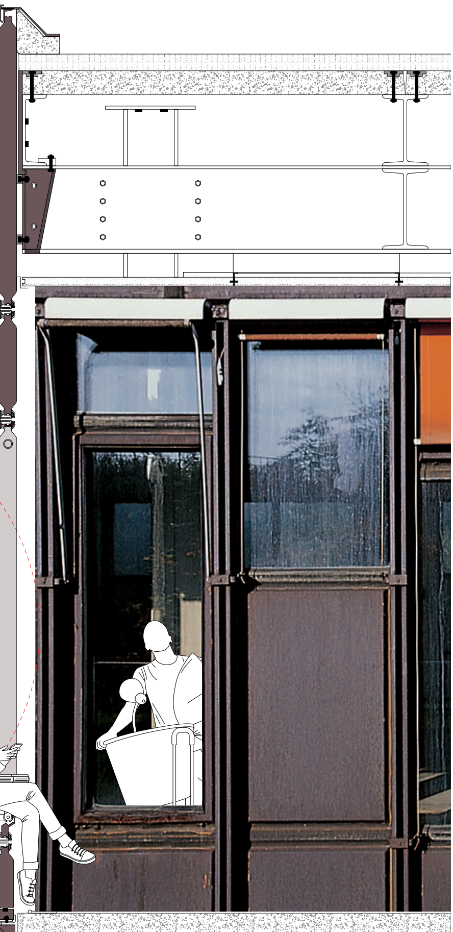
Arquitectura Viva, Library and Restoration of the Free University, Berlin Original Corten-Steel Panels; Jean Prouvé, 1965-1973 Restored in Bronze; Foster + Partners
